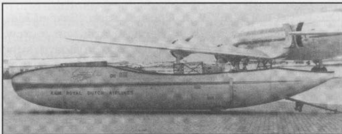
KLM used a number of "Speedpacks" not only for cargo, but also to transport flesh cut flowers to North America. (via Harm Hazewinkel)
