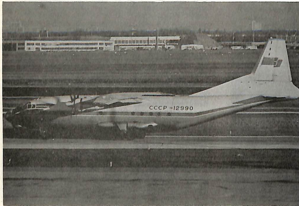
Cargo workhorse of Aeroflot is the demilitarized AN-12, a C-130-type aircraft. Photo at Amsterdam in 1972. Gerritsma files.
