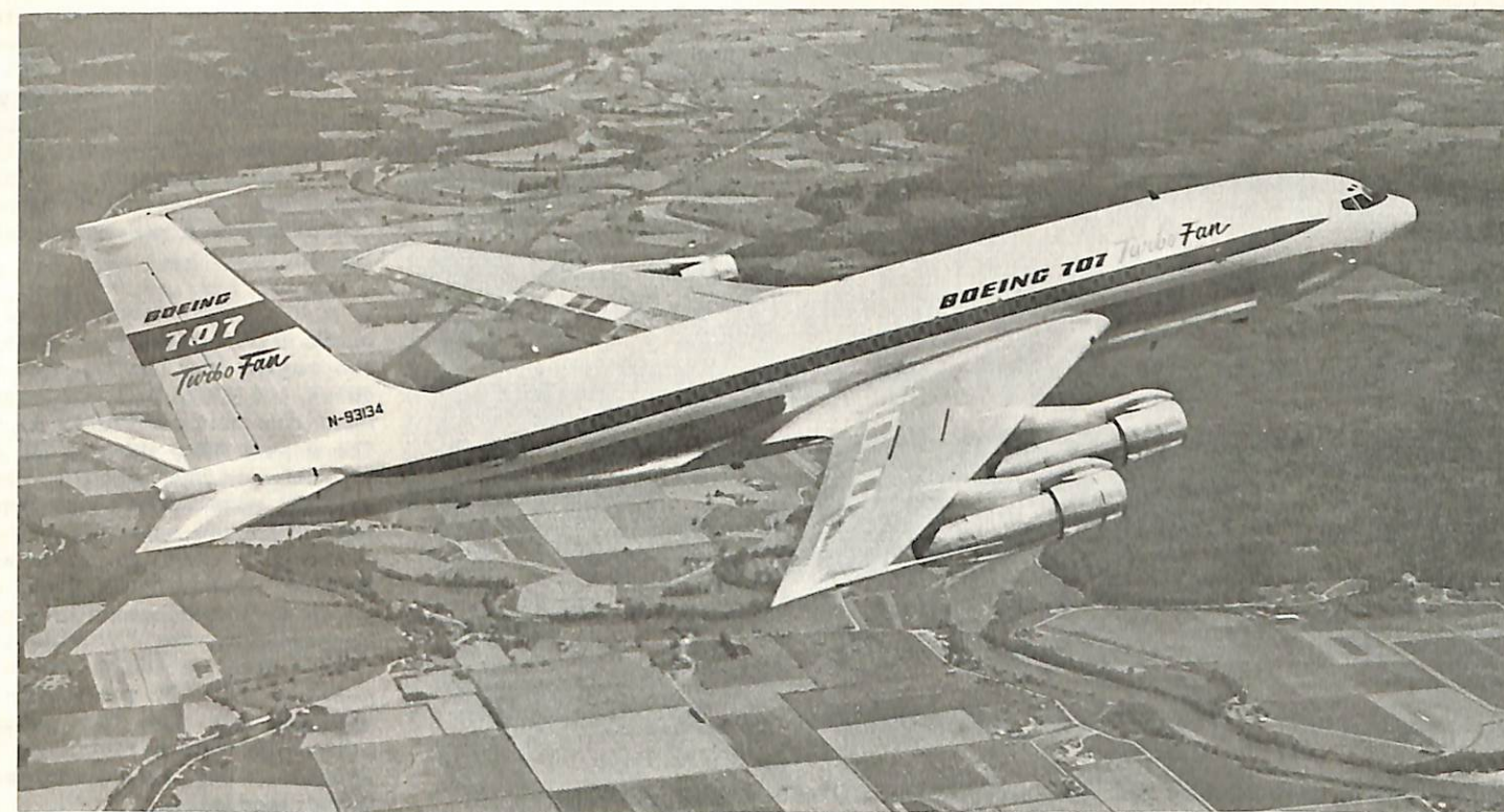
This is the first 707-120B equipped with the Pratt-Whitney turbofan engines. The improvements in performance over the 707-120 were dramatic. Boeing photograph, via Bob Woodling.
