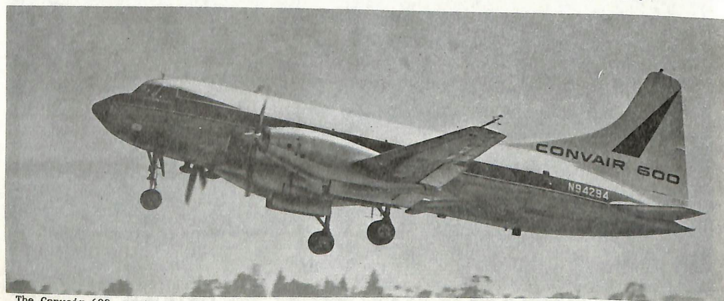
The Convair 600, equipped with Rolls-Royce Dart engines. Convair photo from collection of Tom Kalina.
