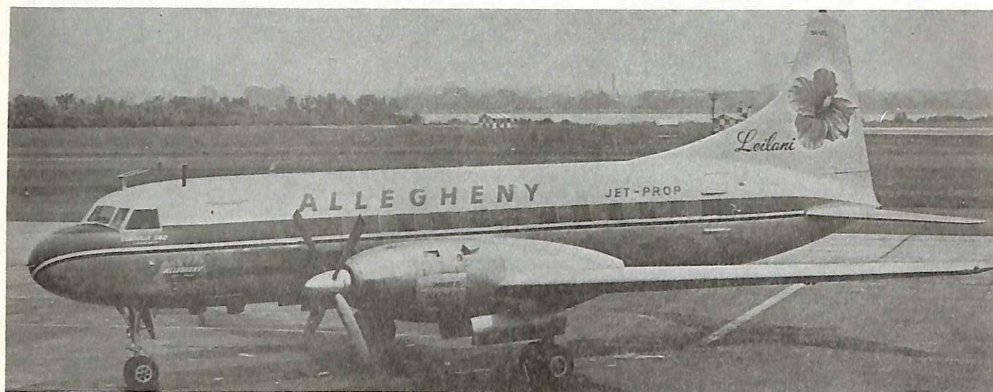
The Convair 540, equipped with the Napier Eland engines. World Airline Hobby Club file photograph.
