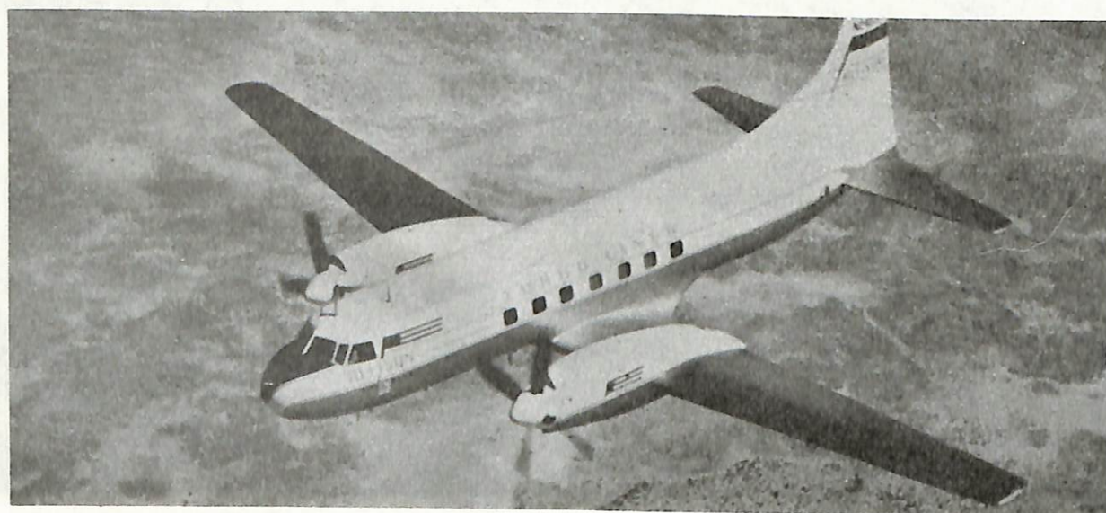
The Convair 580, equipped with Allison 501 engines. World Airline Hobby Club photograph.
