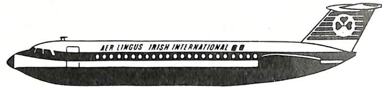
BAC—One-Eleven : 74 passengers, two Rolls-Royce Spey turbofan engines each developing 10,600 lbs thrust. Cruising speed 550 m.p.h. at 25,000 feet.
