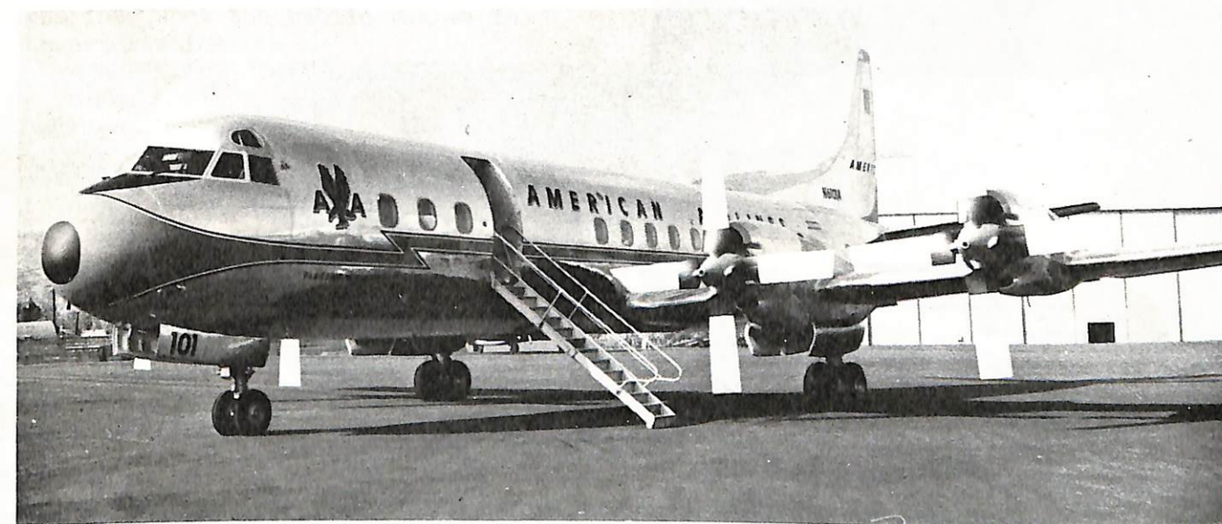
American Airlines L.188 with airstairs extended. When the stairs were extended as shown in this photo, the door would roll into the top of the aircraft.
