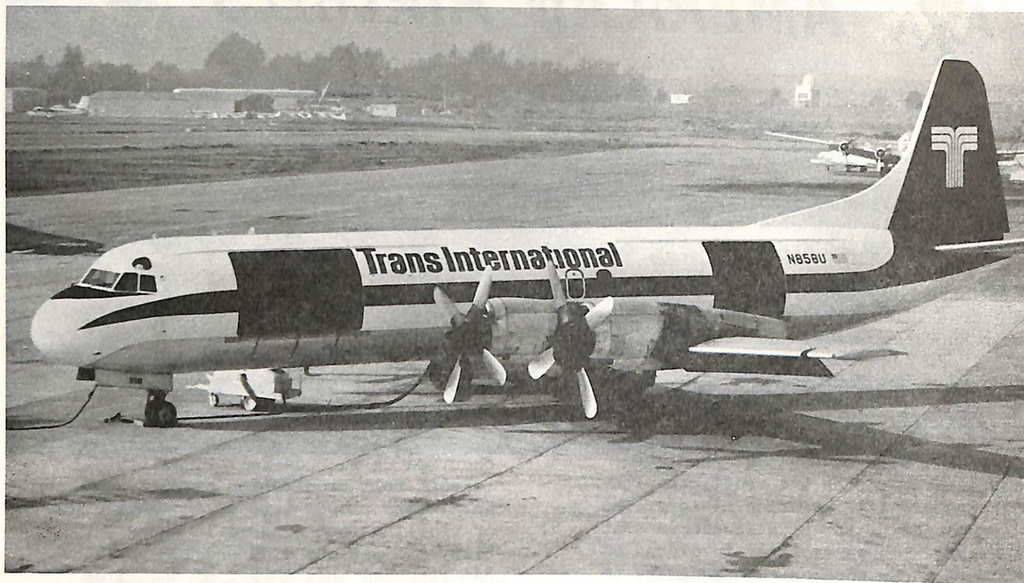
ABOVE: A Trans International Airlines L.188C Freighter. This is a former KLM Electra (ex-PH-LLH). Note large cargo doors and "rounded props." Lion Films photo.
