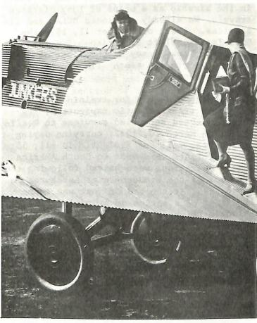
An advanced design for its time, the Junkers F 13 even provided enclosed accommodation for passengers. The plane was covered by a corrugated metal skin and became an important transport aircraft in the 1920s and 30s.
