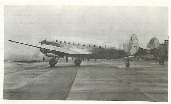
Photograph of prototype CW-20 with twin-tails. Photo from the files of Fred Erdman.
