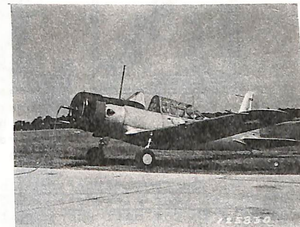
Consolidated BT-13 with pick-up rope attached.
