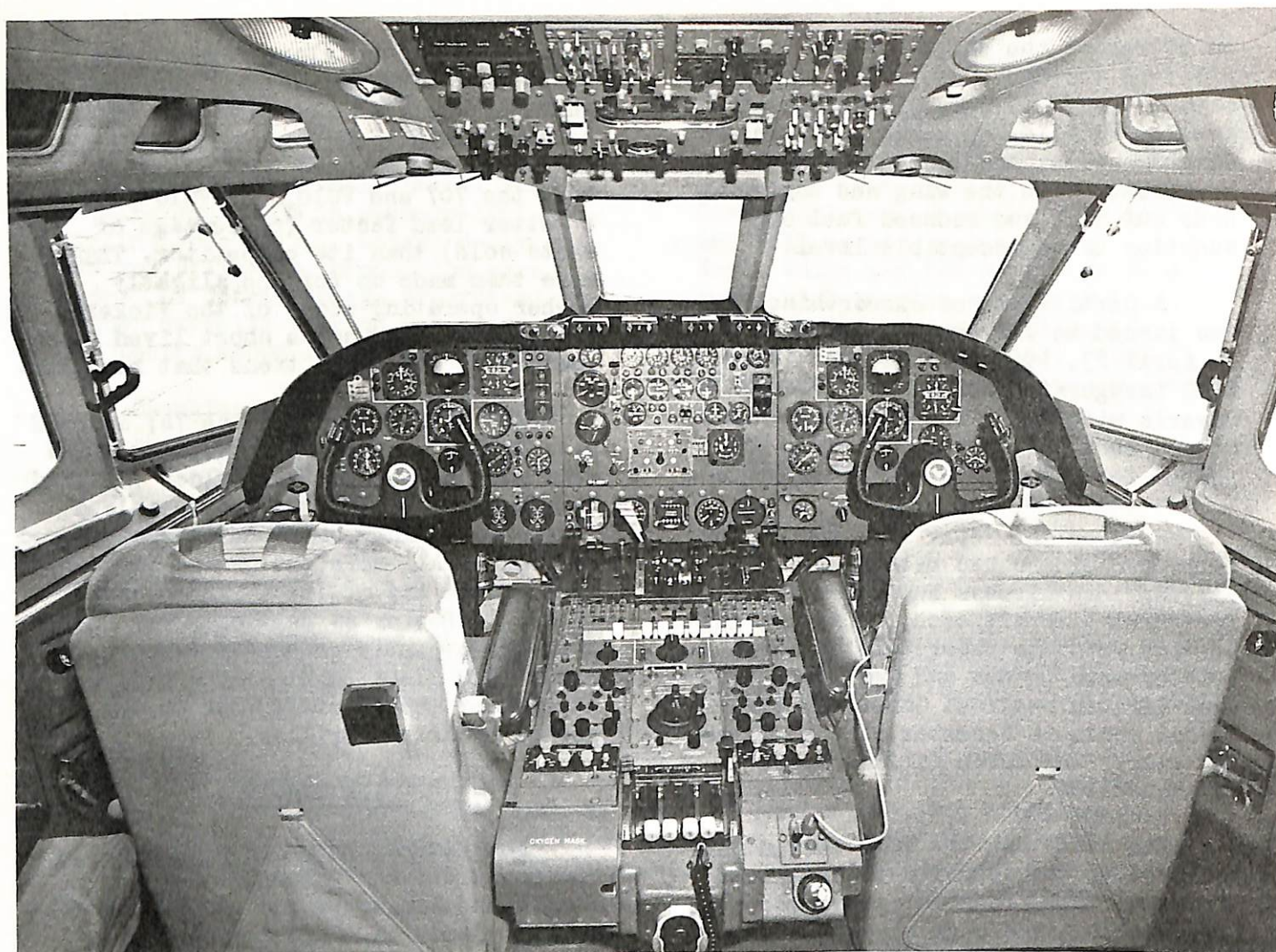
Super VC10 Flight Deck: The Super VC10 flight deck is renowned for its spaciousness and simplicity. The instruments and controls are so arranged that the two pilots can give their whole attention to flying the airplane while a flight engineer looks after the engine and system controls. British Aircraft Corp. photo.
