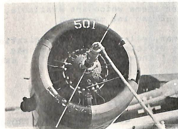
Detail of pick-up attach point on prop hub of BT-13.
