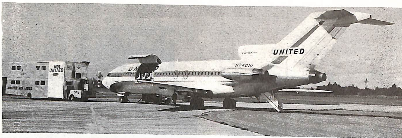
A United Air Lines Boeing 727QC and the van which has been, specially designed for seat transfer and storage while the aircraft is flying on cargo work
