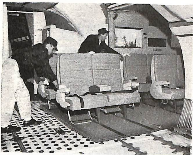
Below, once the fuselage of the 727QC is clear, the loaded cargo pallets can be brought aboard from a loader and pallet transporter which has replaced the storage van. Eight cargo pallets can be loaded and locked down in about 20 minutes (see last week's issue, page 9)
