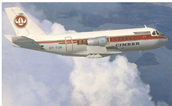
Cimber Airlines VFW 614, OY-TOR. Postcard issued by the manufacturer VFW-Fokker, probably in 1975. The small 44-seat VFW 614 was the first jet aircraft designed specifically to serve the regional airline market. It entered commercial service with Cimber Air of Denmark in late 1975. The aircraft was ahead of its time, and only 16 examples were sold -- to three small European carriers and the German Air Force. (See 'Stateside with the VFW 614' by William F. Mellberg, in Airliner World, October 2015, pp. 58-62).
