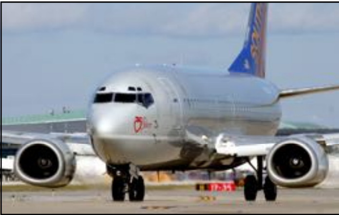
Closeup of Southwest Boeing 737-300 showing the flatter engine nacelles. Photo by Joe Fernandez .
