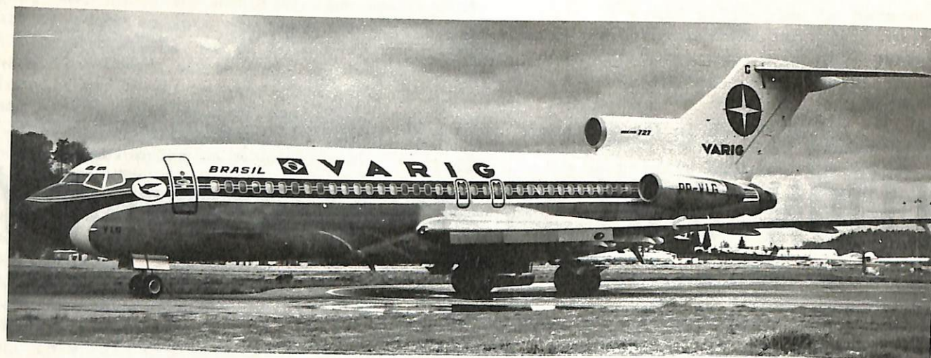
Spanking new PP-VIG, one of nine 727s in VARIG'S fleet, in 1970. Note main gear center doors in open position. These doors normally open only in flight at time of gear extension or retraction.
