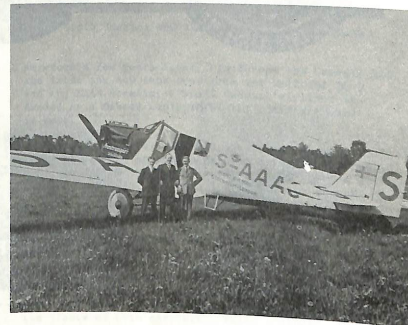
ABOVE: In Sweden, ABA started service with six Junkers F-13 all-metal aircraft for four passengers in an enclosed cabin. SAS photo.
