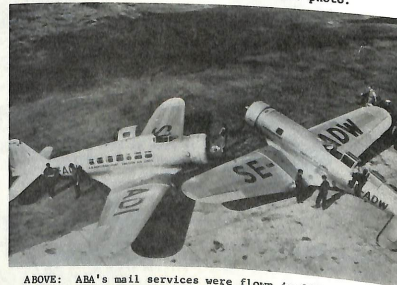
ABOVE: ABA's mail services were flown in 1939 by these two Northrop aircraft, SE-ADI being a Delta C-1 and SE-ADW a Gamma. Gerritsma photo.
