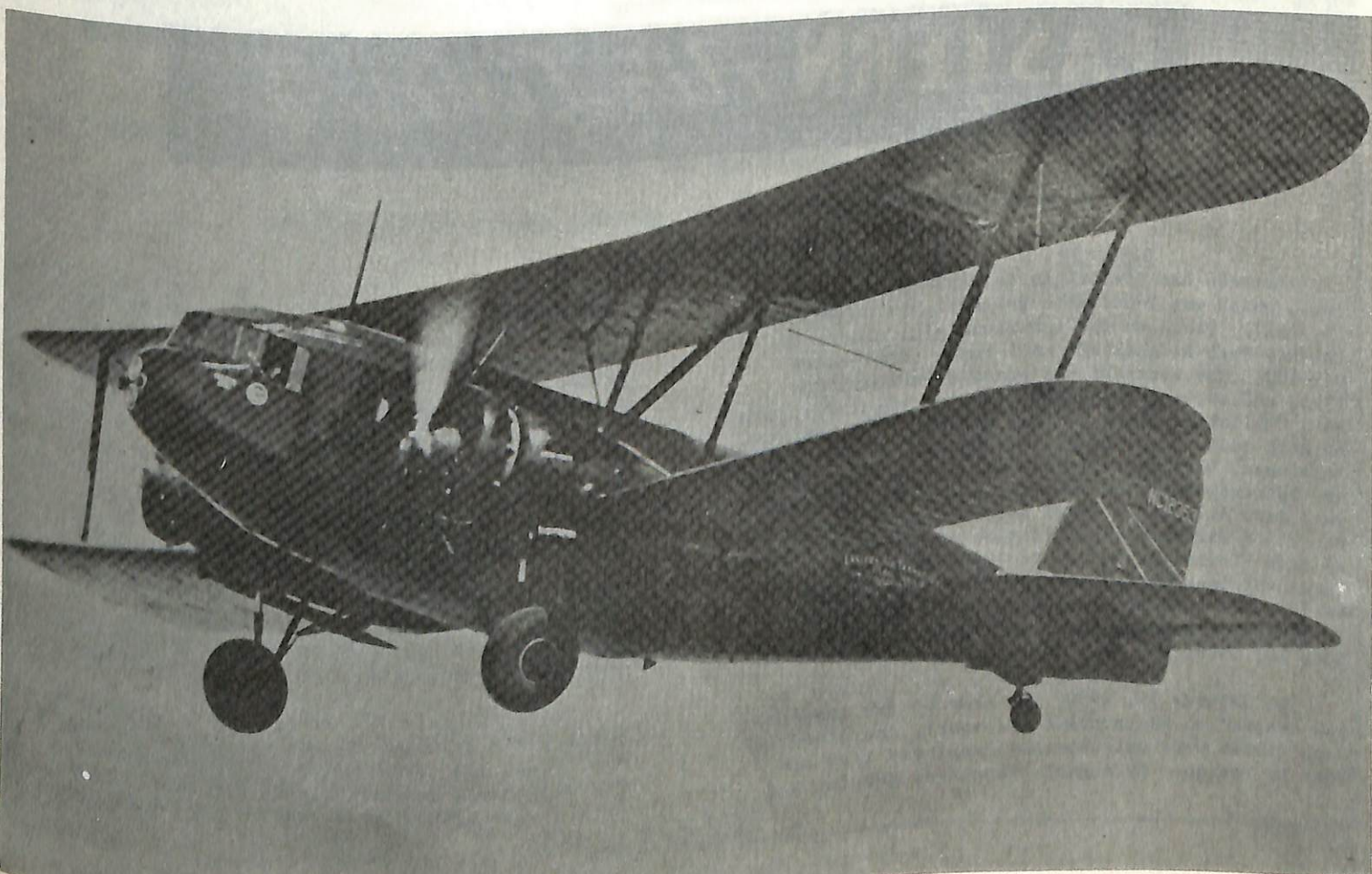
ABOVE: Curtiss CONDOR using liquid-cooled Curtiss Conqueror engines. Aircraft could carry 21 passengers at a speed of 120 mph. BELOW: An advanced Curtiss CONDOR having radial, air-cooled engines. I'm not sure, but I believe these aircraft were painted all dark blue with red/orange lettering. Photos from WAHC files.
