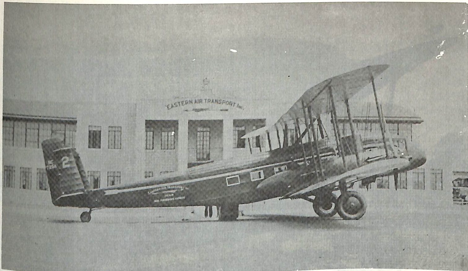
ABOVE: Curtiss CONDOR using liquid-cooled Curtiss Conqueror engines. Aircraft could carry 21 passengers at a speed of 120 mph. BELOW: An advanced Curtiss CONDOR having radial, air-cooled engines. I'm not sure, but I believe these aircraft were painted all dark blue with red/orange lettering. Photos from WAHC files.
